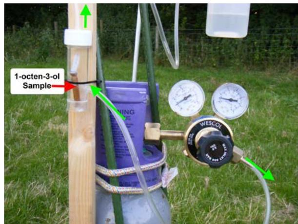
(c). CO<sub>2</sub> Multistage Regulator and Odour Mixing Chamber
