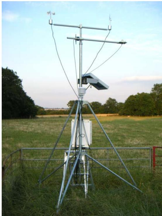
**Figure 5.2.** Automatic weather station with CR800 Measurement and control system (Campbell Scientific Inc., Shepshed, UK) *in situ* at farm A
